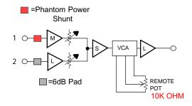
The Model MX414 has one mic input, and one line input, mixed to a common output. Both inputs have adjustable gain. The line input gain range can be increased by 6dB by removing push-on shunt at JP3.
