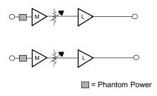
The Model MX413 has two discrete microphone preamplifier channels. Both channels have individually adjustable gain.
