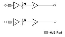
The Model MX412 has two discrete line amplifier channels. Both channels have individually adjustable gain, The input gain can be increased by 6dB by removing pushon shunts (jumpers) at JP2 and JP3. Both inputs and outputs are electronically balanced. They may be used in either a balanced or unbalanced configuration. Requires low voltage AC power (See MXT-1).
