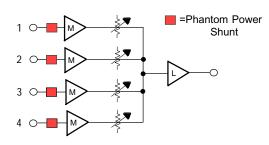
The Model MX409 has four microphone inputs, mixed to a common line output. Each microphone input has 15 volt phantom power circuitry, which is activated by a push-on shunt (jumper). All inputs have adjustable gain.
