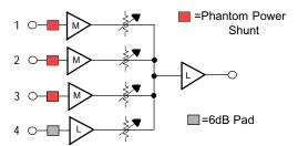
The Model MX408 has three microphone inputs, and one line input, mixed to a common line output. Each microphone input has 15 volt phantom power circuitry, which is activated by a push-on shunt (jumper). The line input has a 6dB pad, which is also activated by a push-on shunt. All inputs have adjustable gain.
