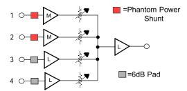
The Model MX407 has two microphone inputs, and two line inputs, mixed to a common line output. Each microphone input has 15 volt phantom power circuitry, which is activated by a push-on shunt (jumper). The line inputs have a 6dB pad, which is also activated by a push-on shunt. All inputs have adjustable gain.
