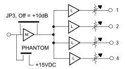
The Model MX405 has one microphone input and four line outputs. The microphone input incorporates a 15 volt phantom power circuit, which is activated by a push-on jumper. The input gain can be increased by 10dB by removing push-on shunt at JP3. The outputs have adjustable gain.
