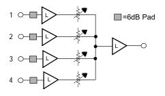
The Model MX404 has four balanced line inputs, mixed to a common line output. Each input has adjustable gain, and a 6dB pad. The pad is activated by placing the RED push-on shunt, on the appropriate connector. The MX404 is shipped with all four pads in place.
