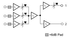
The Model MX403 has three line inputs, mixed to a common signal, and distributed to two line outputs. All inputs, and output #1 have adjustable gain. The input gain can be increased by 6dB by removing push-on shunts (jumpers) at JP2, JP3, and JP4.
