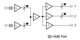
The Model MX402 has two line inputs, mixed to a common signal, and distributed to three line outputs. Both inputs, and outputs 1 and 2 have adjustable gain. The input gain can be increased by 6dB by removing push-on shunts (jumpers) at JP2 and JP3.
