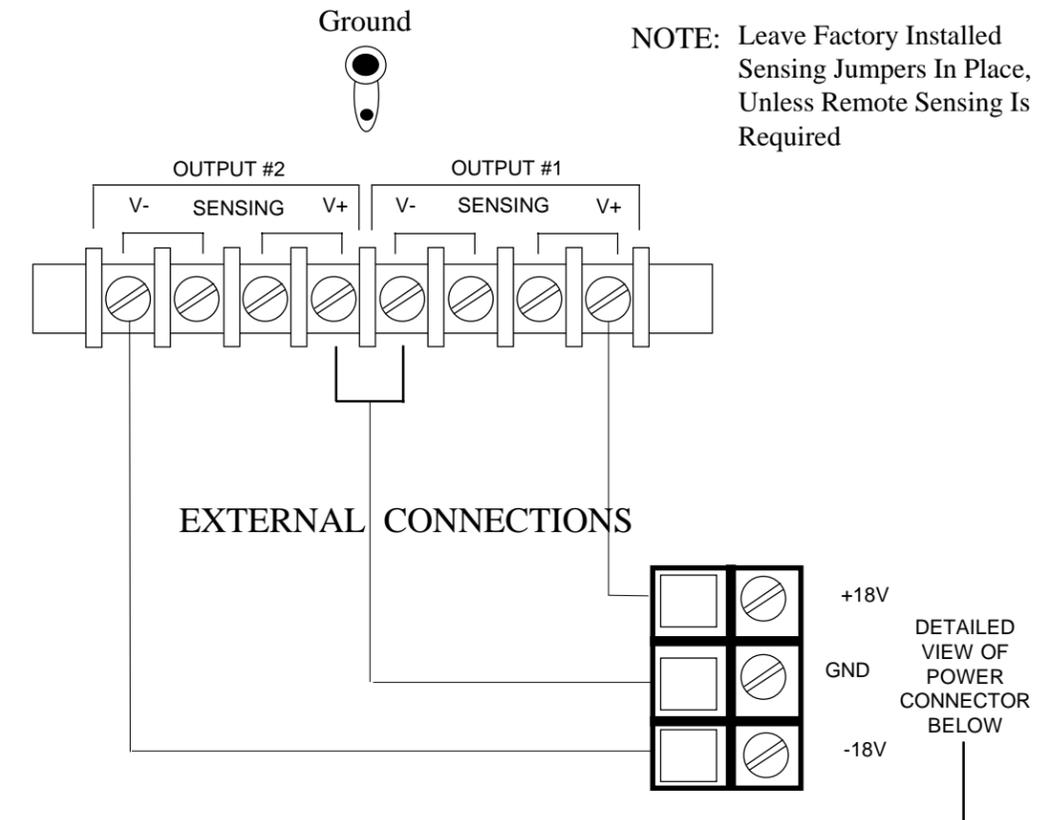
**Power Supply Output is floating with respect to ground. It may be necessary, depending on the individual installation, to provide a ground strap from the card frame "GND" pin to power supply ground.**
