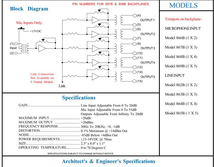
The distribution amplifier shall be constructed as a plug-in printed circuit The distribution amplifier shall contain (2 to5) outputs. Each output shall board module. It shall be designed to allow up to 10 modules to fit in a rack mount card frame, requiring no more than 3.5 inches of vertical rack space. The distribution amplifier shall be unpluggable from the front of the card frame, without the need to disconnect wires attached to the rear connector.
