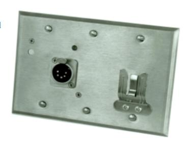
The Protech Audio Model 5053B Remote Microphone Station is designed for use in professional paging and communications systems. The unit is designed to amplify microphone level signals at the source, and prevent the serious degradation of signal-to-noise ratios normally found when microphone level signals are carried over long distances. Typical installations include airport terminals, mass transit stations, convention centers, ball-rooms, arenas, industrial facilities, and theme parks.
